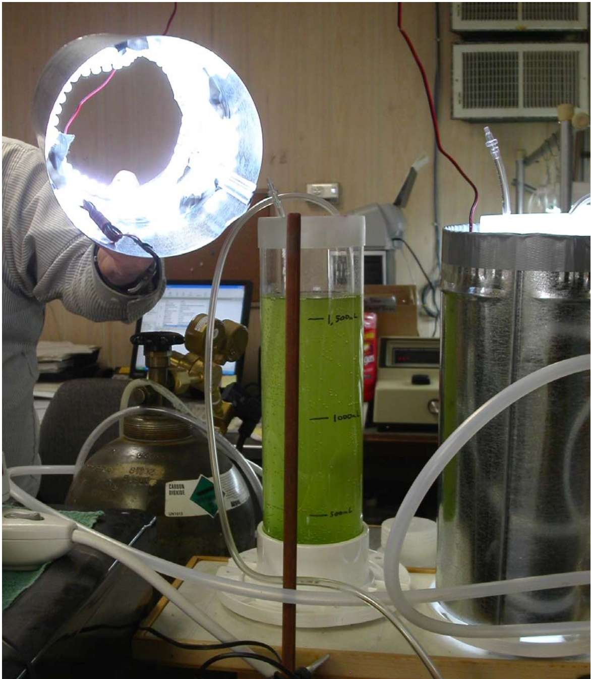
Photo bioreactor (PBR) showing LED light source in a spiral pattern on the internal side of the tubular photo shield.
